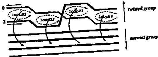
Figure 3: Current loops due to signal line 2 and ground line 0.
